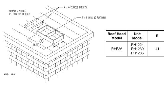
(1) A SEPARATE METAL FLASHING SHOULD BE INSTALLED AROUND WOOD CURBING. CAULK & SEAL ALL JOINTS & WEATHERPROOF.
